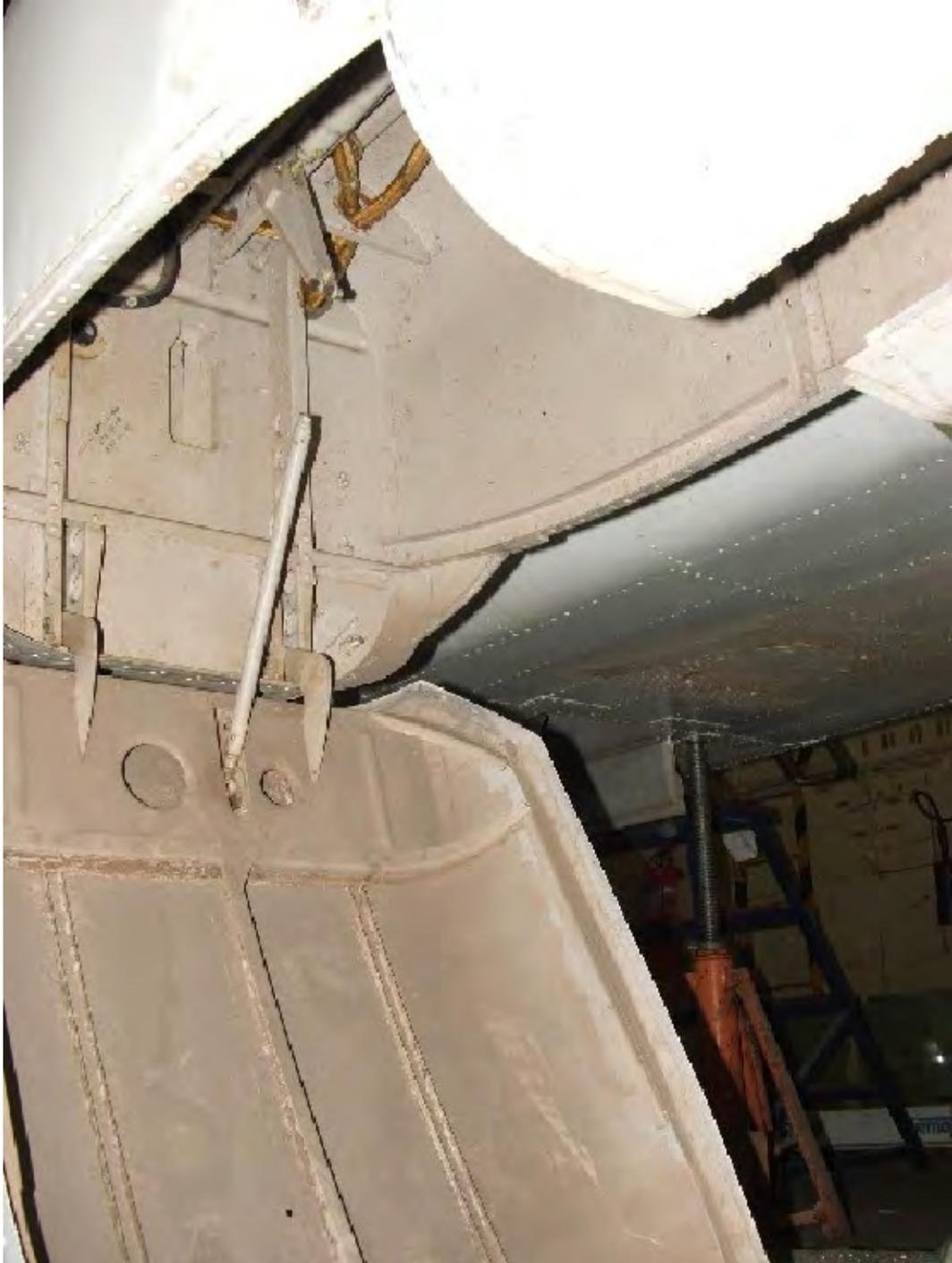
**Figure 1 LH Landing Gear Pod Door - Disconnected (RH Similar)**
