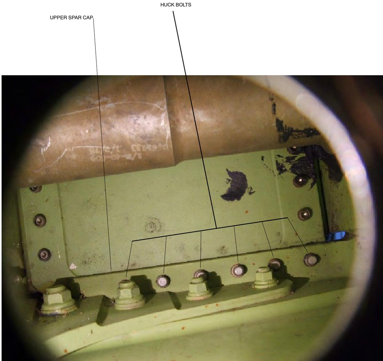
**Figure 6 Upper Spar Cap Viewed through Inspection Hole**
