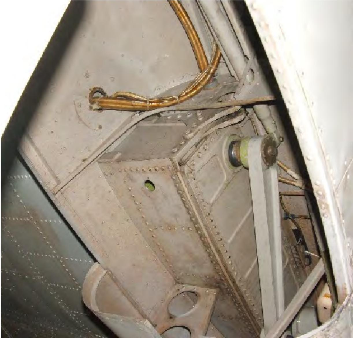
**Figure 2 LH Stub Wing Inspection Hole (RH Similar)**
