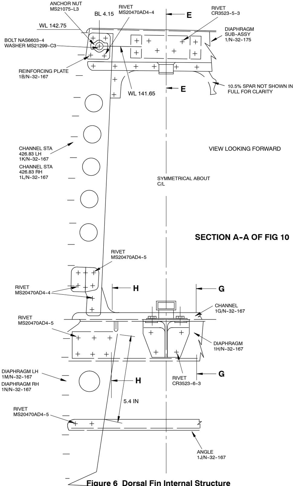
**Figure 6 Dorsal Fin Internal Structure**
