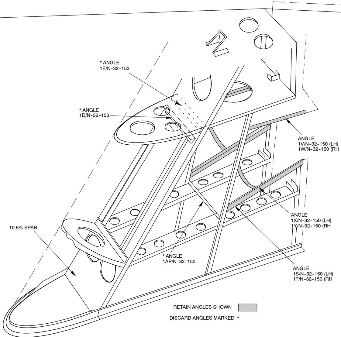
Figure 5 Dorsal Fin Internal Structure (Pre-Mod N663)
