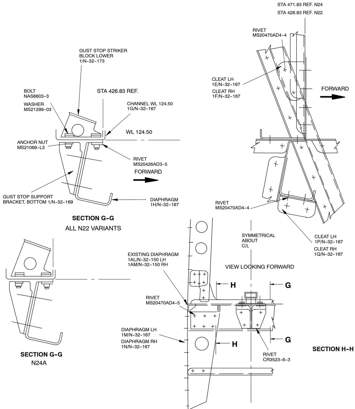
Figure 9 Channel Installation
