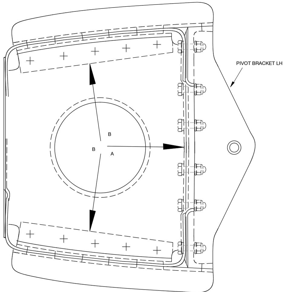
**Figure 1 Cross Section of Horizontal Stabiliser Centre Section Showing Inspection Views**
