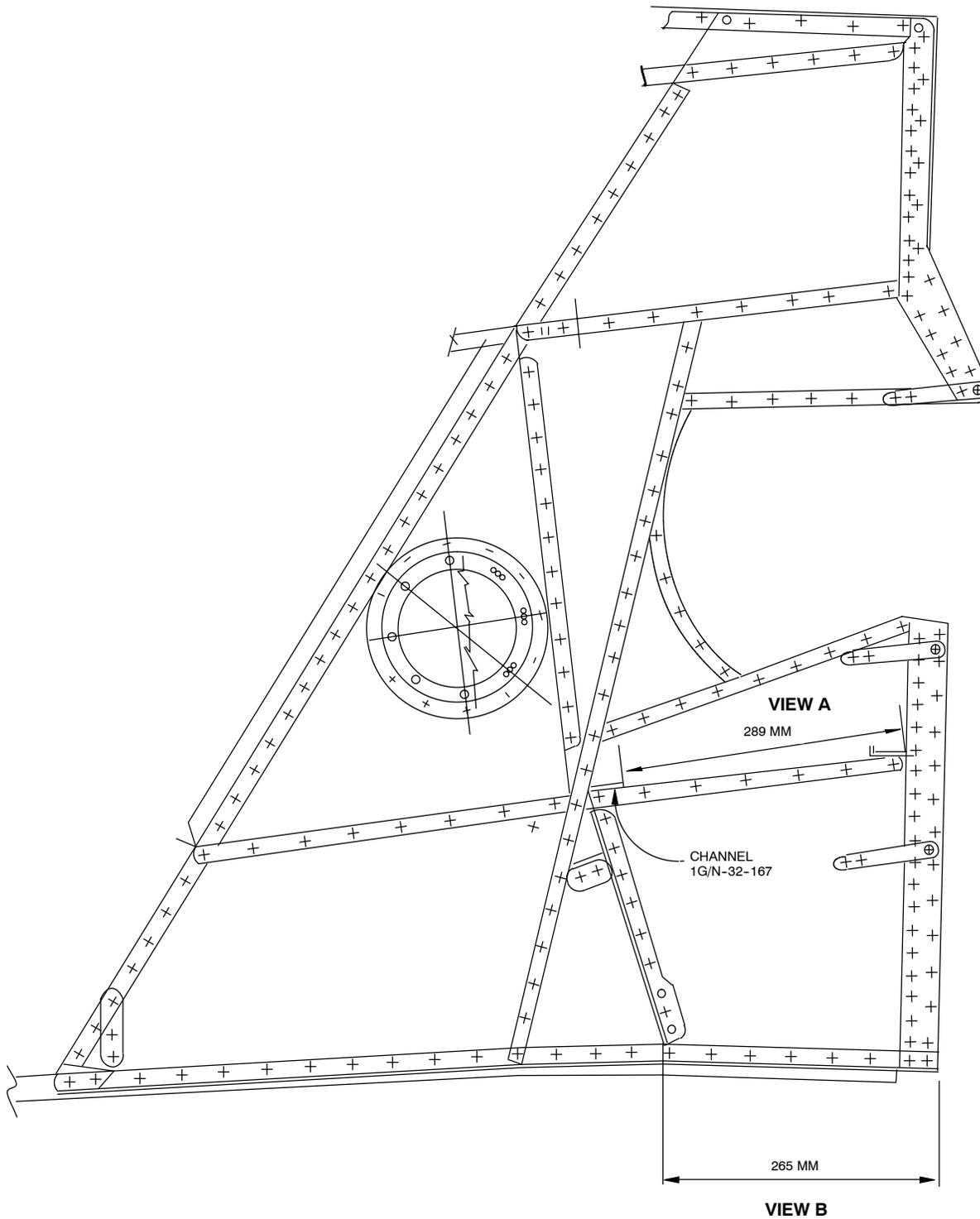
Figure 8 Diaphragm Installation
