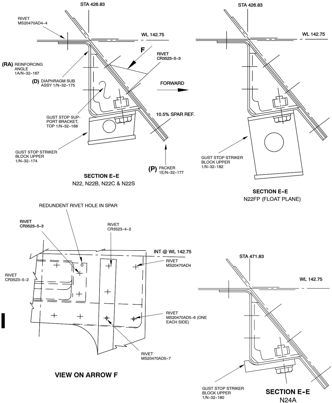
Figure 7 Gust Stop Support Bracket Assembly — Upper
