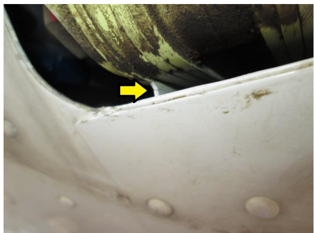
Figure 4: Typical Cracks Images courtesy of aircraft operators
