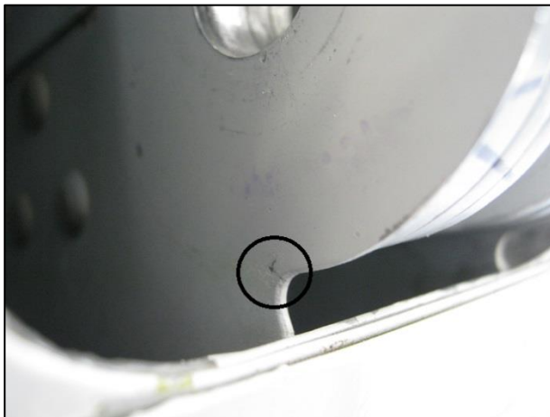
Figure 4: Typical Cracks Images courtesy of aircraft operators
