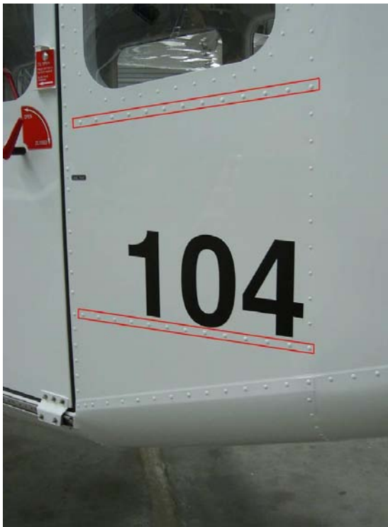
Figure 2: Remove 2 rows of rivets below aft windows L & R.
