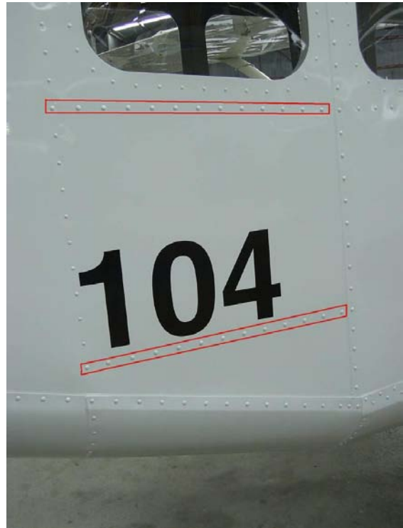
Figure 2: Remove 2 rows of rivets below aft windows L & R.
