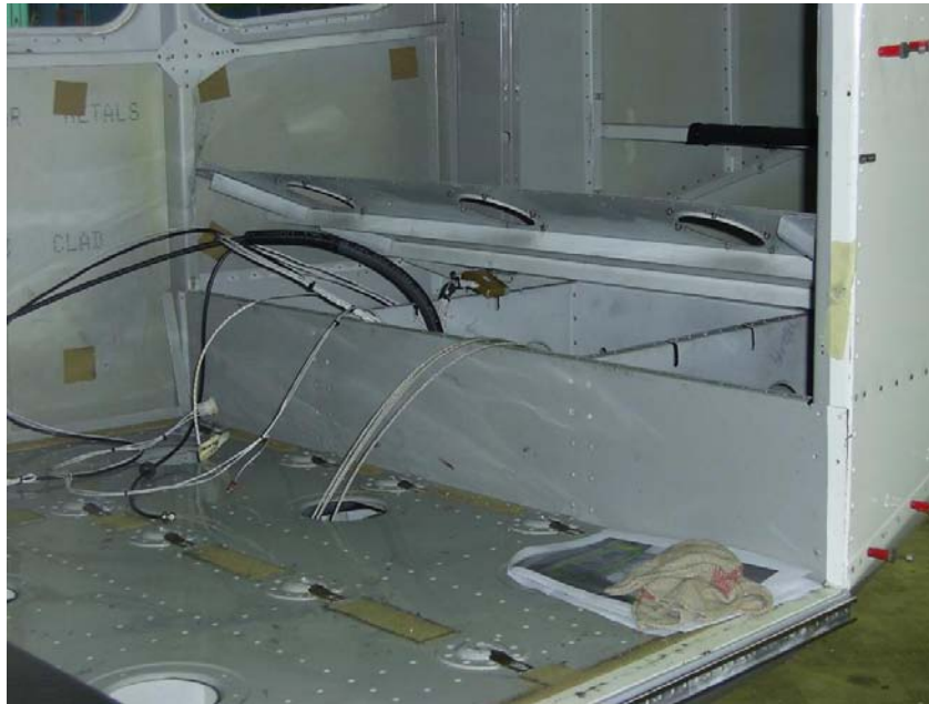
Figure 7: To gain easy access to area under Baggage shelf release shelf skin from left and right sides by easing baggage shelf bulkhead forward, shelf skin can then be raised to allow access to rivets on aft flange of shelf ribs as above picture. The shelf will not be able to be removed from the cabin before the tailcone is removed.
