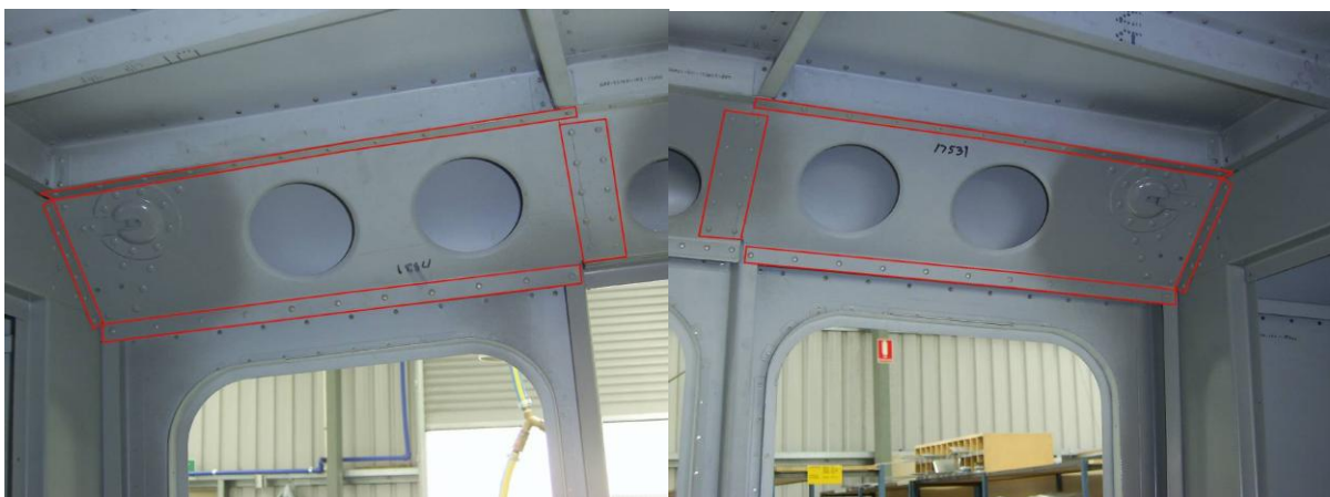
Figure 1: Drill out rivets outlined from Upper L & R cornice panels.
